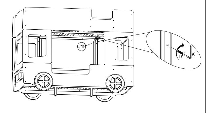
Step 14.Use Hex Key(K)to tighten the Ladder Connect Bar(C24)to the Ladder Left Side Tube(C22)and Ladder Right Side Tube(C23)with Bolt(G).
