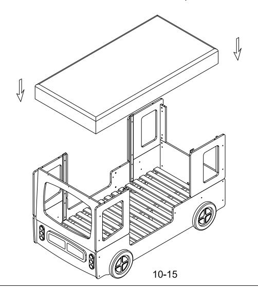
Step 9.Insert the Nut(F)to the Top Headboard Panel(C13)and Top Footboard Panel(C14); Use Hex Key(K)to tighten the Top Right Side Rail(C3)and Top Left Side Rail(C4)to the Top Headboard Panel(C13)and Top Footboard Panel(C14)with Bolt(F).
