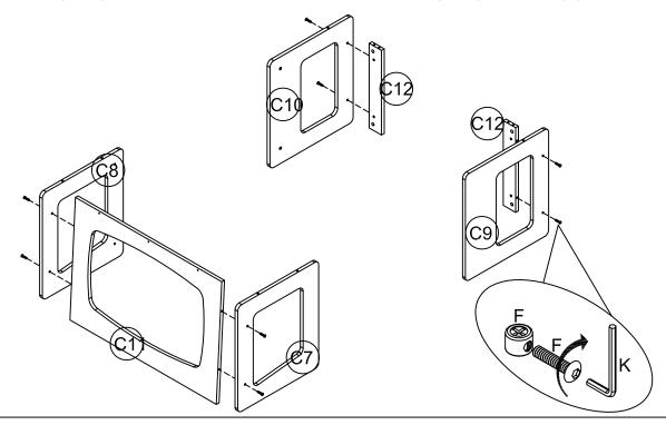
Step 4,Assemble the Bottom Headboard Window Panel(C11) and Right Side Connect Panel(C7,C9) and Left Side Connect Panel(C8,C10) to the Right Side Rail(C1) and Left Side Rail(C2), Use a Phillips Head Screw driver to assemble the Bottom Headboard Front Panel(C5) to the Bottom Headboard Window Panel(C11) with Bolt(I).
