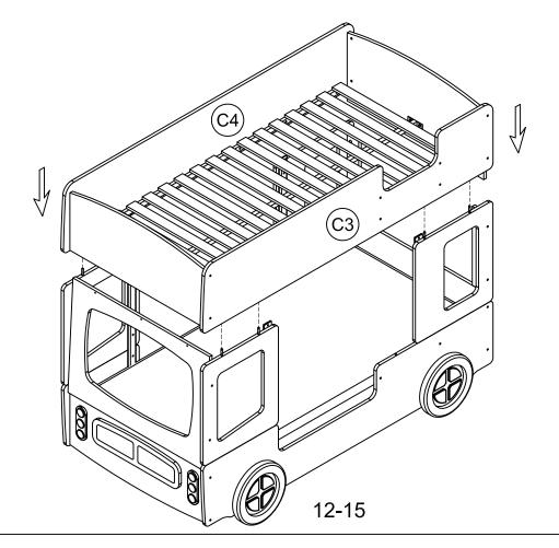
Step 13.Use Hex Key(K)to tighten the Top Right Side Rail(C3)and Top Left Side Rail(C4)to the Connect Tube(C19)with Bolt(D).
