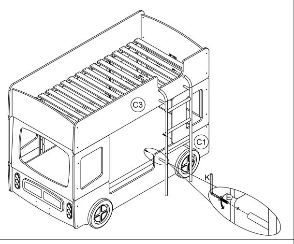
Step 16.Use a Phillips Screwdriver to assemble the Licence Panel to the Bottom Headboard Front Panel with Screw(J), Insert the Mattress.
