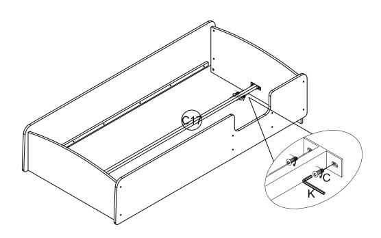
Step 11.Use a Phillips Head Screw driver to tighten the Slats(C18)to the Top Right Side Rail(C3)and Top Left Side Rail(C4) with Bolt(I).
